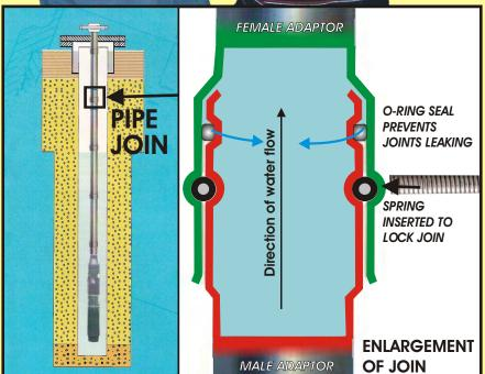
The push-on coupling pipes are available in 6m and 3m lengths. Compromising lengths are available in 2m and 1m.
